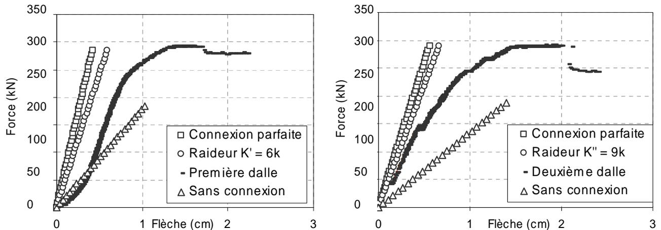
Figure 7. Results of two bending tests on two slabs (left, width 400 mm and 6 lines of connectors, right, width 300 mm and 9 lines of connectors).
