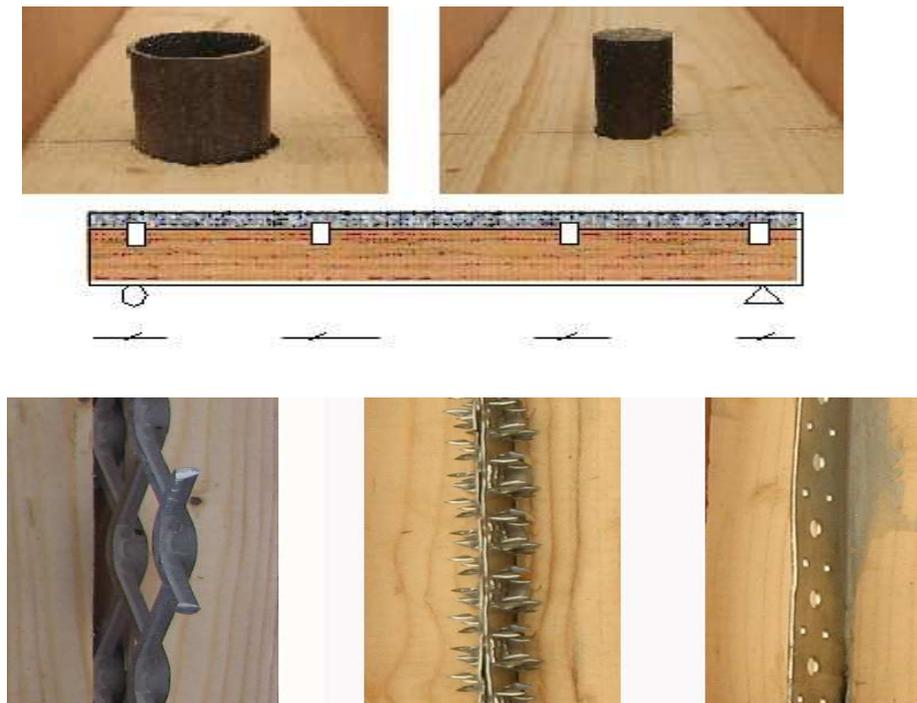
Figure 1. Examples of connectors (from left to right and top to bottom) Tube (PTu), Rod (PTi), Expanded metal (PMD), spike plate (PPAP), Perforated strip (PR).
