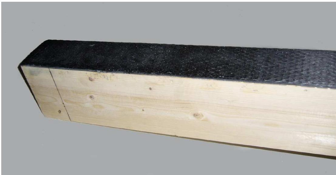
Figure 8. Example of a glulam beam reinforced with vacuum-glued fabric (ENPC)
