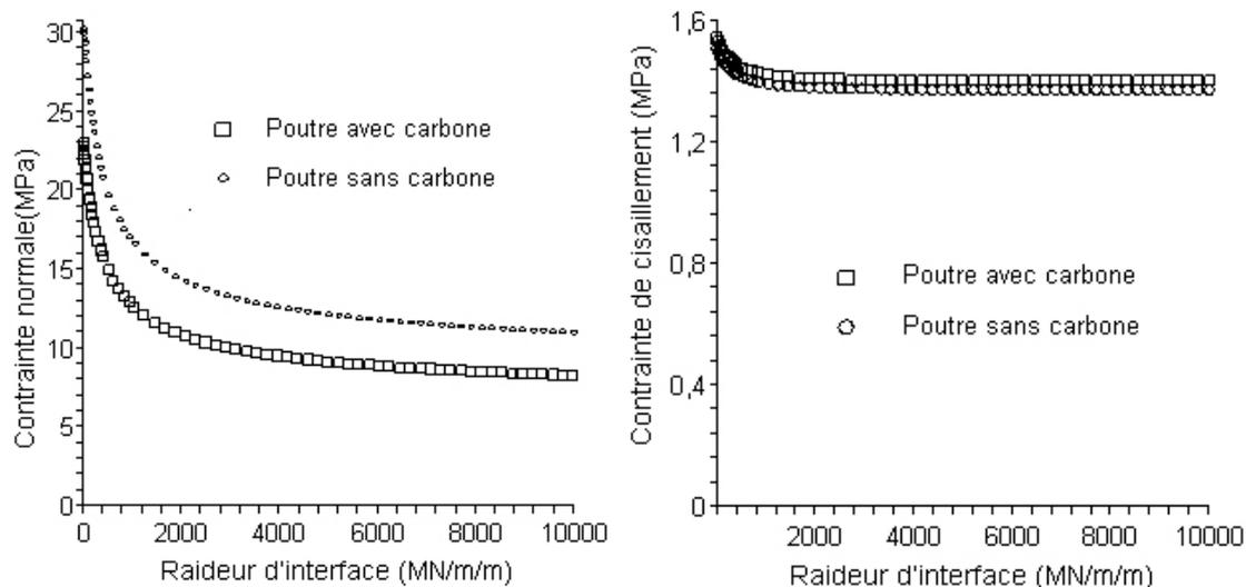
Figure 10. Development of normal stresses (on the left) and maximum shear (on the right) in the wood as a function of the stiffness of the wood-concrete interface. Big square points are relative to reinforced beam with carbon, small diamond shaped points are relative to non reinforced beam.
