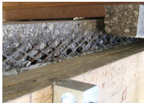
Figure 9. Load versus slipping at the interface on end and shear failure in the concrete.
