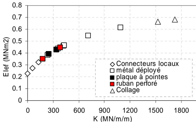
Figure 5. Stiffness  $(EI)_{ef}$  as a function of the interface stiffness  $K$  as per the EN 1995-1-1 model for the values of  $(EI)_{ef}$  measured.
